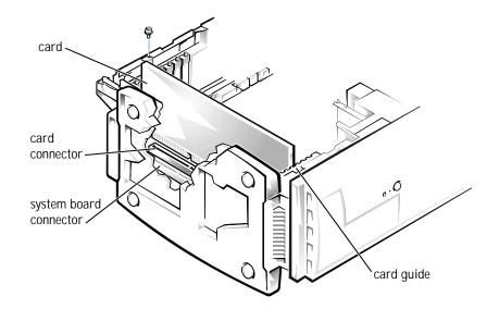
Make sure that the card is fully seated and that its bracket is within the card slot.
