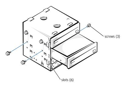
9 With the slots on the drive cage extending slightly beyond the front of the computer, lower the drive cage and slide it toward the back of the computer until the cage locks into place. 10 Connect a power cable to each drive.
