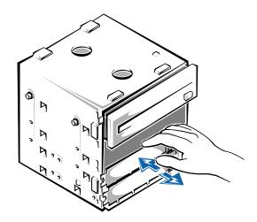
9 To install a new drive in the lower 3.5-inch bay, slide the drive into the bay and secure it with three screws.
