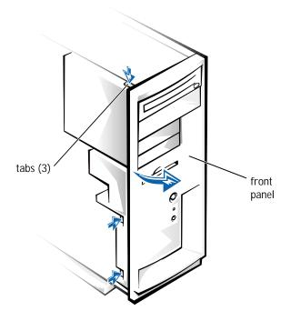
HINT: You must remove the upper insert to remove the lower insert.
