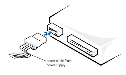
• NOTICE: When you attach the extra connector to the new drive in the following step, match the colored strip on the cable with pin 1 on the drive.
