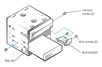
HINT: Be sure to remove the 1/4-inch screw on the right side of the drive cage.
