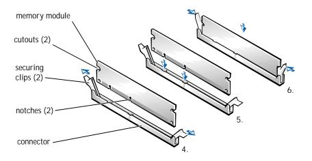
To remove a memory module, press out the securing clip at each end of the memory connector until the memory module disengages from the connector. 7 Replace the computer cover (see page 71).
